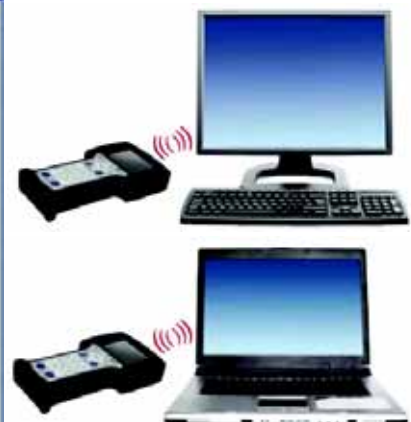
FIGURE 4. Easy Upgrade allows communication between the 375 Field Communicator and a PC using IrDA. The IrDA port enables transfer of configuration data and upgrades between the 375 and AMS Device Manager.
